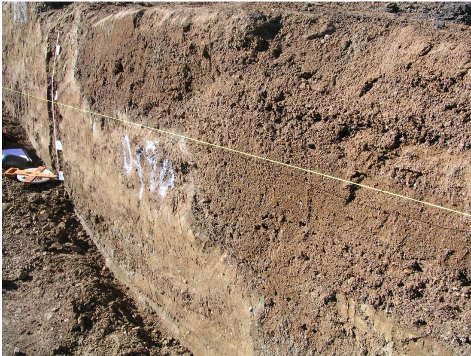
Figure 6. Channel fill next to the reddish paleosol that was in Soil Paleosol No. 2 (vertical tape) in the north wall of Trench FT-2.
