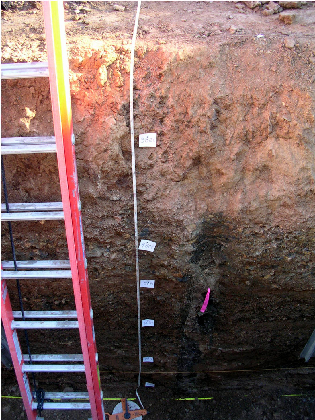
Figure 2. Lower portion of Soil Profile No. 1 at Station 0 + 43 in the south wall of Trench FT-1 west of the West Beverly Hills Lineament, which lies east of Beverly Hills High School. Clay film development reaches over 440 cm in this profile.
