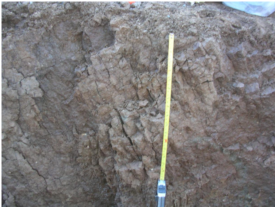
Figure 7. Tilted prismatic and angular blocky soil structure within the paleosol on the south wall of Trench FT-2 across from Soil Profile No. 3. The tilting is a result of soil creep that occurred when an active channel existed immediately to the east.
