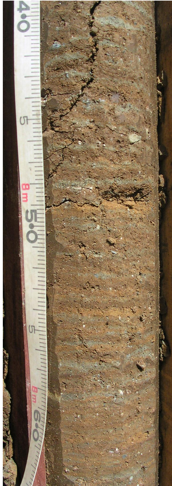
Figure 9. Varves in Soil Profile No. 6 (core boring CB-13) reflecting seasonal redox conditions produced when high rainfall formed a marsh at this locality. The term “varve,” once used exclusively for glacial lakes, is now used for other fluctuating fresh-water environments.
